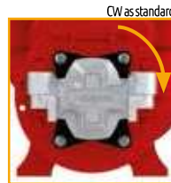
Version H MEC 9000: Group 3.5 51.83 cc/rev - Pmax 230 bar - In G 1" - Out G 1" MEC 11000: Group 3.5 73.82 cc/rev - Pmax 180 bar - In G 1" - Out G 1"1/4 MEC 13500: Group 4 86.56 cc/rev - Pmax 280 bar - In G 1"1/4 - Out G 1"1/2
