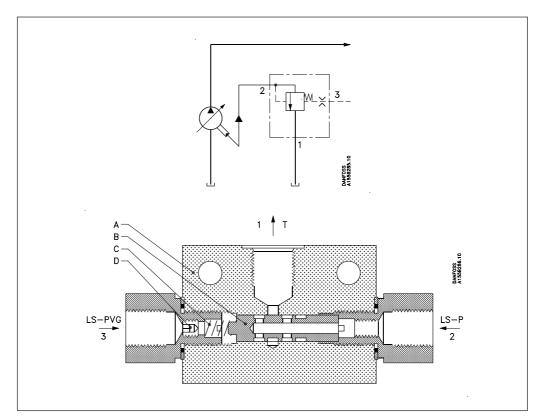
LS-PVG: Connection to LS-port, PVG LS-P : Connection to LS-port, pump Tallene 1, 2 og 3 are stamed into the valve housing A: Housing B: Spool
