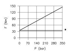
\* In ECD solenoid valves, pressure in chamber 1 is uninfluential and the necessary force to make the override working is 35 Nm.
