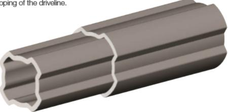
The dimensions of the "Four-Tooth" profile are the largest possible within the space available between the ears of the yoke.
