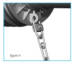
Close clip (figure 4) and replace the screw.
