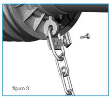
Fit the chain and reposition the clip (figure 3).
