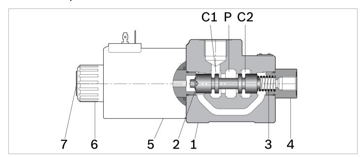
A valve basically consists of a housing (1), a control spool (2), a return spring (3) and a solenoid (5). It is designed to select which one of two circuits (C1 or C2) is to be supplied with the oil delivered from one single hose (P): with spool in position "0", when the solenoid is de-energized, the flow goes from P to C1, with spool in position "1", when the solenoid is energized the flow goes from P to C2. With the coil de-energized, the return spring (3) pushes
